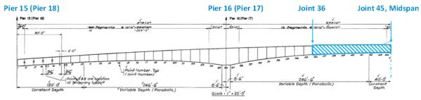
Figure 9: Longitudinal elevation. Pier 15 to the mid-span (the west half).
