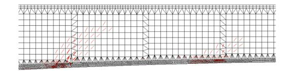
Figure 23: Crack diagram at load factor of 1.0 from a previous analysis
