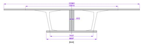
Figure 13: The analyzed I-shape beam cross-section (red) and the original cross-section (dashed line) at segment 12.
