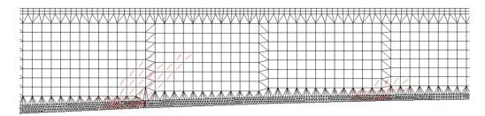
Figure 22: Crack diagram at load factor 0.9 of Phase I.
